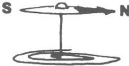
Balance the compass needle on the stand, away from any metal or magnets. It should spin freely. The painted, arrow-shaped end should swing and point north (N). This is the N pole of the compass needle. The other end points south (S). This is the S pole of the needle.
