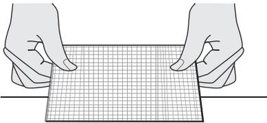
8. Carefully remove the remaining screens from the pulp. Allow the new paper to dry.
