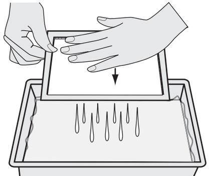
5. Holding one hand on top of the plastic sheet, and the other on the bottom of the frame, flip the frame and remove it. You should now have the screens, pulp, and plastic sheet remaining in one hand.
