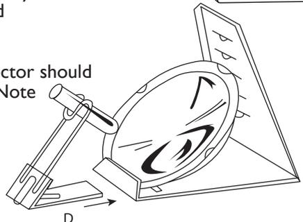
**NOTE:** On a windy day, place some stones or any other suitable weight into the bracket under the reflector, to prevent it from being blown away!
