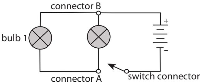
Putting two light bulbs side by side in a circuit like this is called wiring them in parallel.
