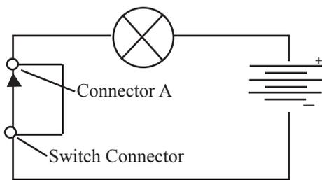
No Short circuit - the wire does not bypass the light bulb. It bypasses the switch, which will no longer break the circuit. The light bulb is always lit.
