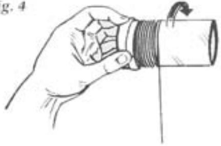
3. When you come to the end of the wire, finish up so that the wire at the beginning of the coil and the wire at the end of the coil are on the same side of the coil tube. Be sure you have at least 3 inches sticking out over the end of the tube. (Fig. 5)
