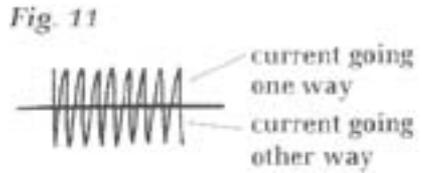
**Fig.11** is one way of illustrating this alternating oscillator current.
