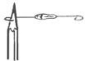
3. Make a small loop at one end of each connecting wire, the same way you did with the diode.
