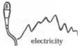
The microphone takes these sounds and turns them into electrical impulses that exactly correspond to the pattern of the announcer's speech, illustrated by **Fig. 10b**. Loud sounds make for strong electrical impulses. Soft sounds make weaker impulses. A diagram of the strengths of the electrical impulses would match up with the sound diagram exactly.
