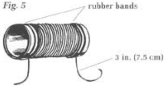
4. Slip another rubber band over the tube and wire to hold the end of the wire in place. Make sure your coils are neat and tight, and put the tuning coil aside.
