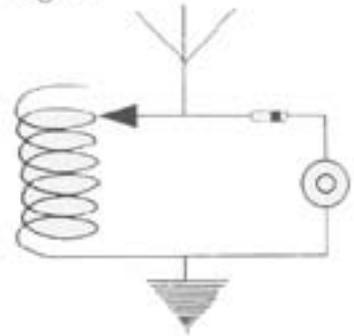
Compare this circuit diagram with the earlier sketch of the radio. Notice how much simpler the circuit diagram is. But notice how the circuit diagram shows the same essential information as the drawing.
