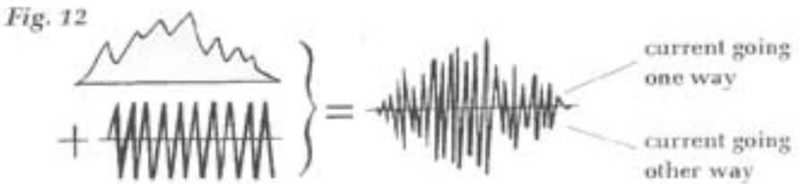
Notice that the bottom half of the new current is a mirror image of the top half. In the top half of the diagram, the current is flowing one way; in the bottom half, it is flowing the other way.
